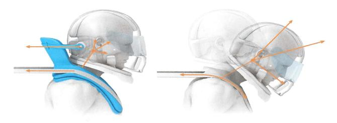
The above sled-test drawings show the HANS at work. With only a neck to restrain it, a 15-pound helmeted head lunges forward at 107 g during a 40-g head-on collision. Resulting "shear" (two opposing forces perpendicular to the neck's axis) and "tension" (pulling force along the neck axis) loads vastly exceed the injury threshold, making death more likely.
